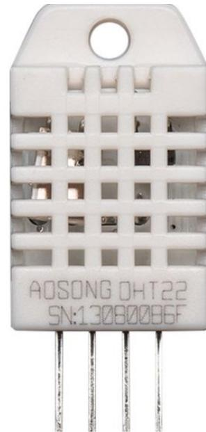
Typically you need a 4.7K or 10K resistor, which you will want to use as a pullup from the data pin to VCC. This is included in the package
