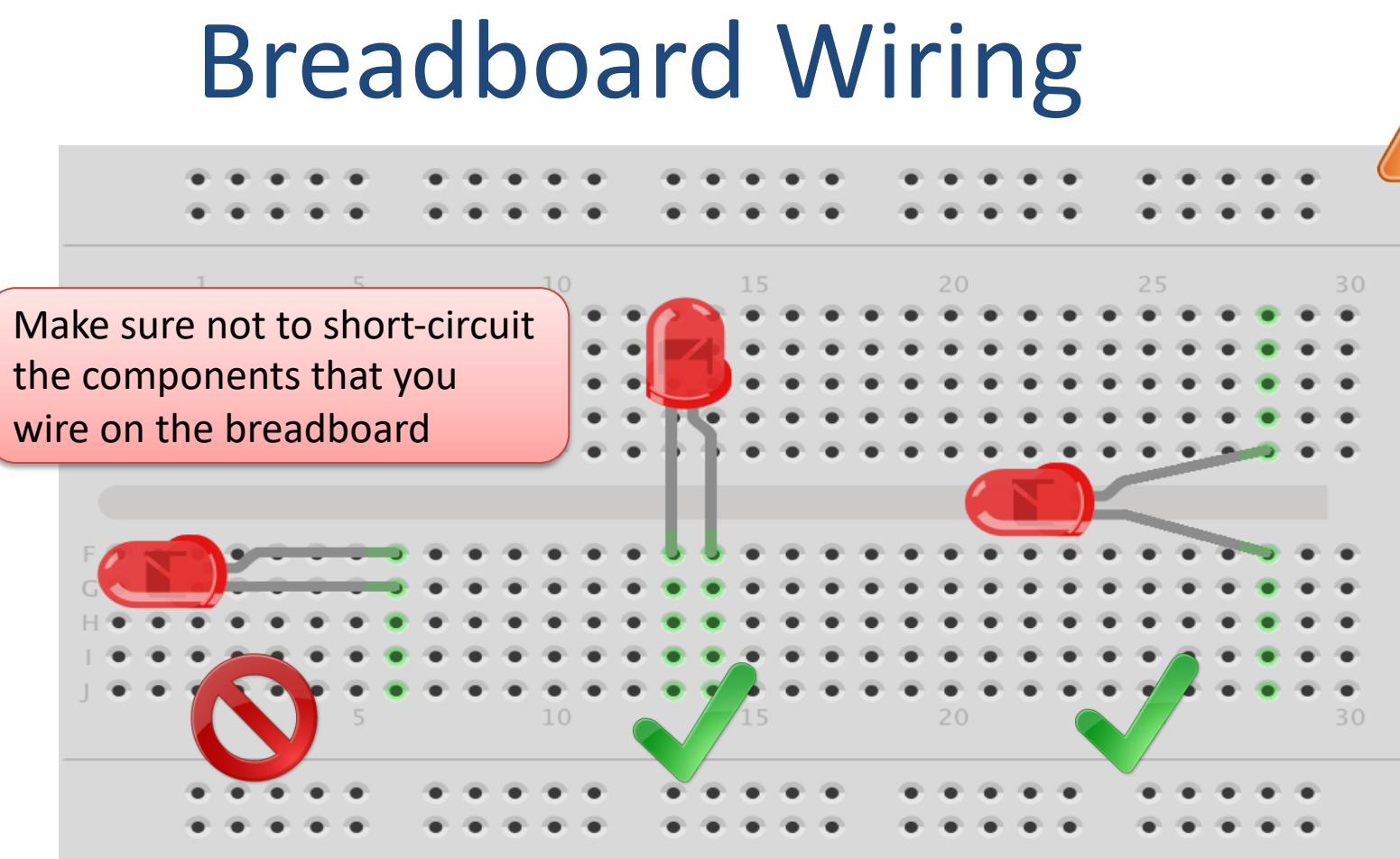
The Breadboard is used to connect components and electrical circuits
