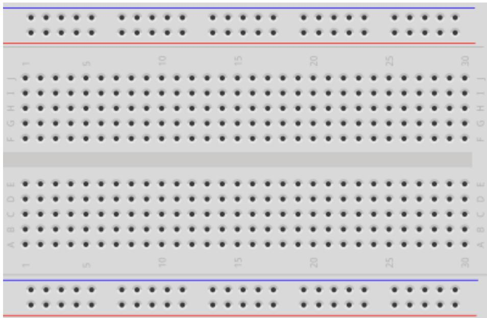
A breadboard is used to wire electric components together
