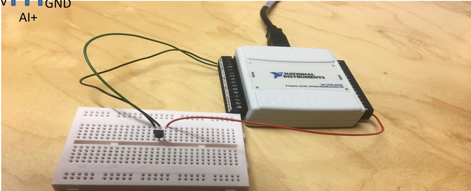
We connect the TMP36 to LabVIEW using a USB DAQ Device from National Instruments, e.g., USB-6001, USB-6008 or similar. I have used a breadboard for the wiring.
