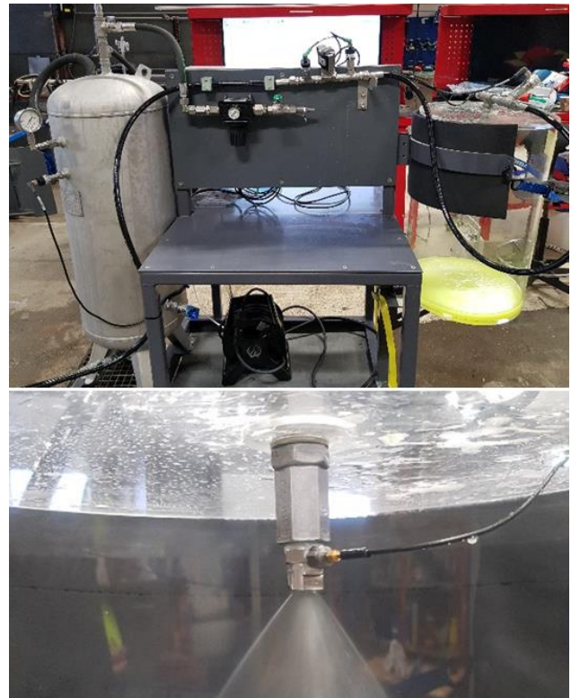
Figure 3. Anti-icing nozzle test rig (top), nozzle with acoustic sensor (bottom).
