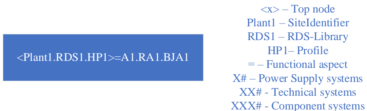
Figure 2: RDS tag in the functional aspect [4]
