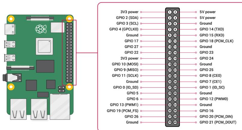
Figure 1.8: GPIO Connector
