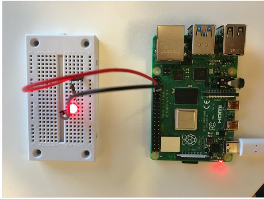
Figure 1.10: LED wiring
