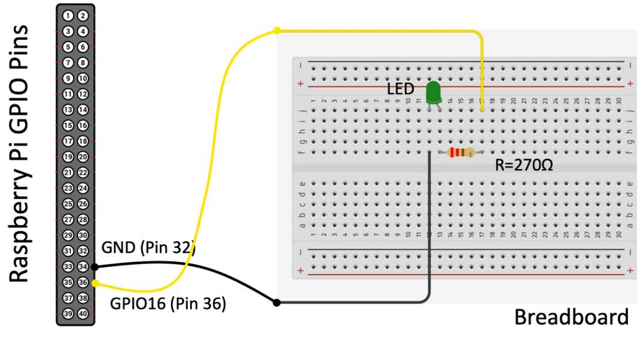
Figure 1.9: LED wiring
