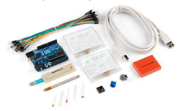
The Arduino platform has 14 digital I/O channels and 6 analog I/O channels.
