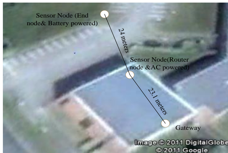
Figure 6.16: Top view of College to show where the sensor nodes and gateway were installed; and their separation distance
